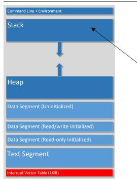
The local variable **sum** is allocated on the stack as would the local variable **i**. However, short-termed variables such as the loop variant **i** are often never allocated in RAM, but instead a CPU register is assigned to implement the variable.
