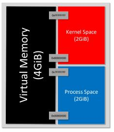
Note the addresses for each space. The *process space* addresses always have a zero in the most significant bit; the *kernel space* addresses always have a one in the most significant bit.
